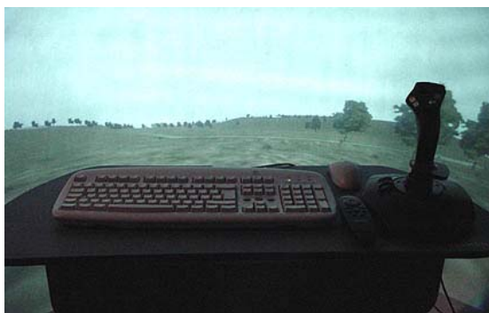
Figure 2: Vision Station and the DVR system written in C++ using VTree and Terravista
