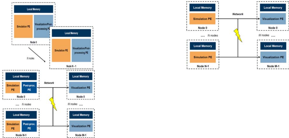
Fig. 1. (a) Tightly coupled approach: visualization and computation shared the same resources. (b) Loosely coupled approach: visualization and analysis run on separate resources. (c) Hybrid approach.
